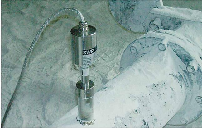
SolidFlow 2.0 is the latest generation of microwave-based measuring systems for measuring the flow of solids.
