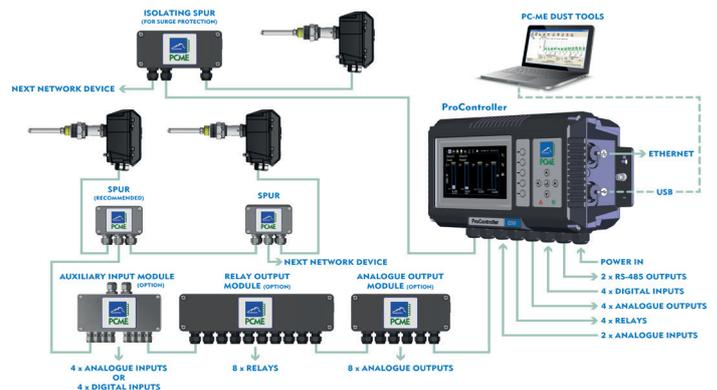
Figure 5: Typical multi-sensor layout
