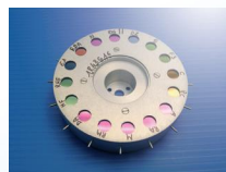
Correlation wheel equipped with optical filter and gas cells
