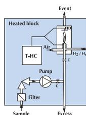
**GRAPHITE 52M-S:** Equipped with one burner placed in a heated block, the GRAPHITE 52M-S allows continuous and accurate Total HC monitoring.
