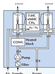
**GRAPHITE 52M-D:** Equipped with two burners and a catalyst, it allows the automatic or manual simultaneous measurement of Total HC and CH<sub>4</sub>. The GRAPHITE 52M-D is ideally suitable to follow transient phenomena during which simultaneous evolution of non methane hydrocarbons and methane.
