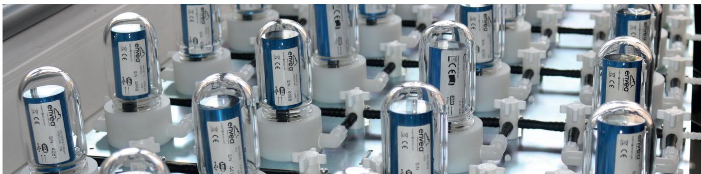
\*Cairsens® are manufactured in France and calibrated in our metrological laboratory using Standard Reference AQMS monitors. Every sensor shipped includes a **calibration certificate**.
