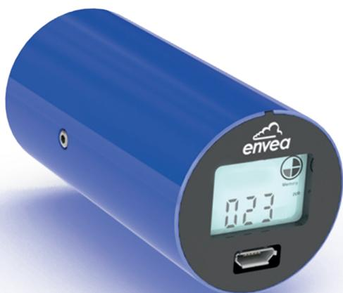
Most of the Cairsens® sensors use amperometric technology consisting of three electrodes: the working electrode (anode), the counter electrode (cathode) and the reference electrode. The gas to be analyzed is diffused through a permeable membrane towards the sensitive electrode. The function of the gas, oxidation takes place at the anode, or reduction at the cathode. The electrical signal generated between the two electrodes is proportional to the concentration.
